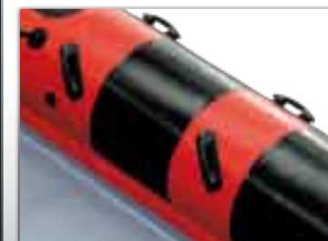
Tube reinforcement and handles (diver)
