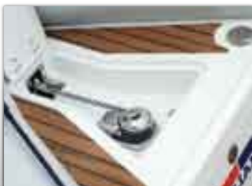
Electric windlass with anchor (on 750 Cruiser only)
